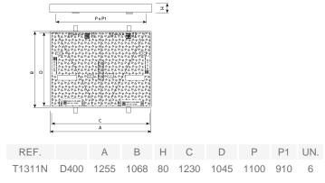
Comunicación is designed to withstand medium traffic. It is perfect for installing on roads with an ADT of 1,000-20,000, particularly road carriageways (including pedestrian streets), stabilised hard shoulders and parking areas for all manner of vehicles.
