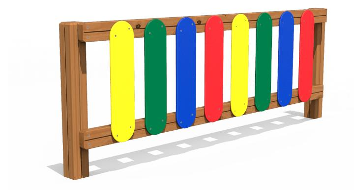
**Structure, Laminated wood:** scandinavian laminated pine wood treated in autoclave Class IV. Finished with two layers of Lasur paint. - In case of being subjected to bad weather conditions, laminated pine wood can present some tiny cracks on the surface that do not reduce its durability at all. As regards resin and knots, please note that these are part of its natural appearance.
