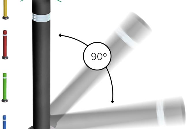
Luminous solar LED bollard made of flexible black polyurethane resistant to UV rays with reflective band. With base plate for a bolt-on installation. Manufactured in fixed and removable version with polyurethane or stainless steel base. Exceeds a flexion of 1500 cycles at 45° and 50 cycles at 90°, without damage.
