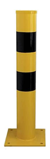
Material: steel, epoxy paint Finish: yellow and black colour Wall thickness: 3.5mm Base plate: 8mm thickness Impact resistance: 16,000 J
