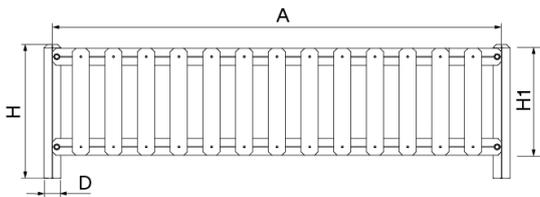
**Structure, Laminated wood:** scandinavian laminated pine wood treated in autoclave Class IV. Finished with two layers of Lasur paint. In case of being subjected to bad weather conditions, laminated pine wood can present some tiny cracks on the surface that do not reduce its durability at all. As regards resin and knots, please note that these are part of its natural appearance.
